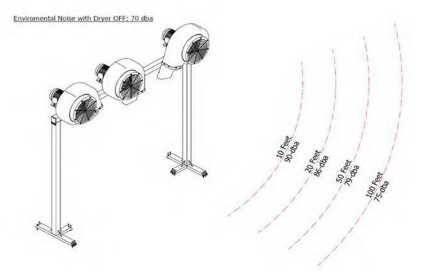
Figure 15. Dryer Noise DBA Reading
